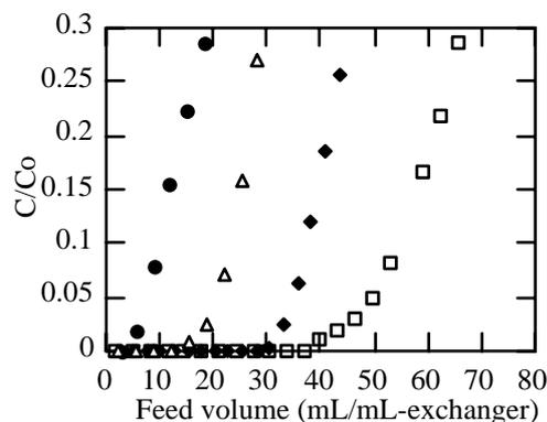
Fig. 1. Breakthrough profiles of  $\text{Cu}(\text{II})$  in column mode uptake of  $\text{Cu}(\text{II})$  by phosphonate fibers and resin. (◆) RCSP  $10 \text{ h}^{-1}$ , (●) RCSP  $500 \text{ h}^{-1}$ , (□) FCPS  $1000 \text{ h}^{-1}$ , (Δ) FCP  $1000 \text{ h}^{-1}$ .
